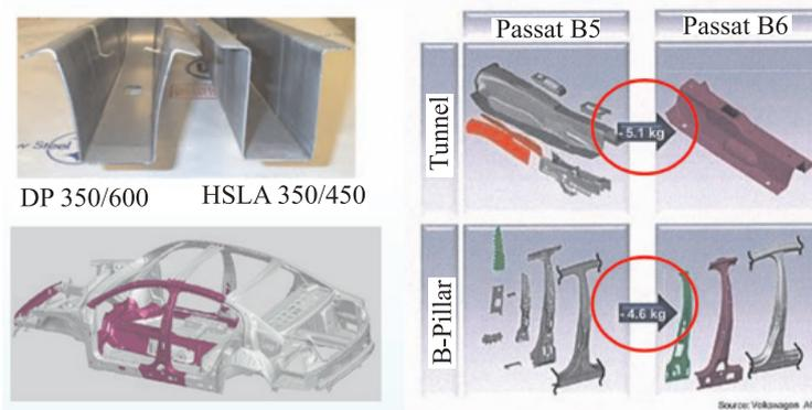
Fig.2. High strength steels in vehicles with improved safety and light weight<sup>(1)</sup>.
