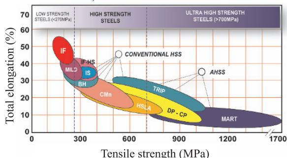
Fig.1. The elongation vs strength of different steel materials<sup>(1)</sup>.
