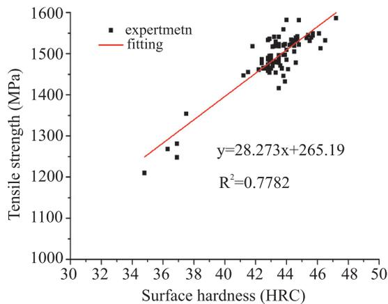
**Fig.18.** Relationship of hardness and strength for hot stamping steel after die quench.
