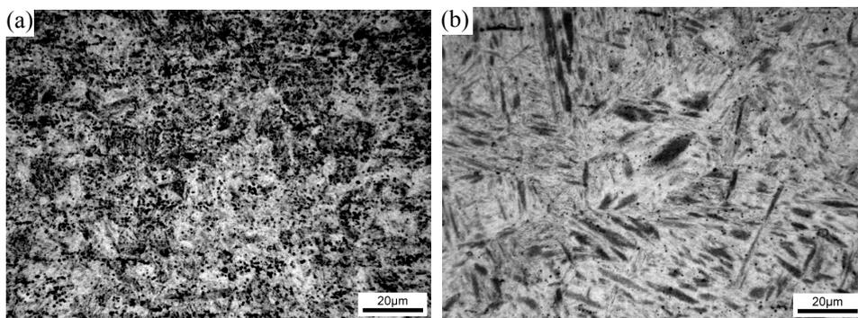
**Fig.17.** The microstructure of 15B22 after die quench from prior heating temperatures (a) 880°C and (b) 930°C.
