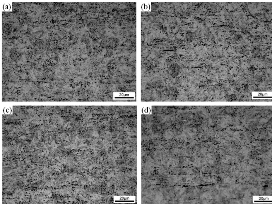
**Fig.15.** The microstructure of 15B22 after heating to 880°C followed by sending the specimen to the mold under 25 tons pressure die quench in time: (a) 5s; (b) 10s; (c) 15s and (d) 20s
