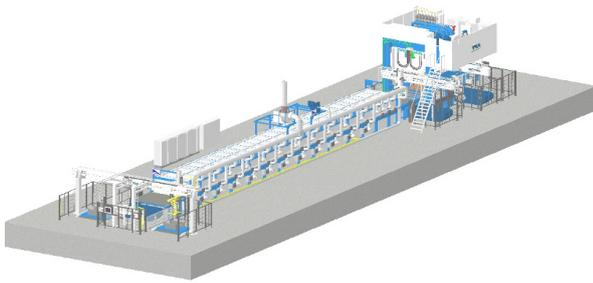
**Fig.5.** Typical hot stamping production line (AP&T Company)<sup>(5)</sup>.
