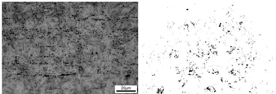
**Fig.16.** The microstructure of 15B22 heating to 880°C and sending to the mold in 20 seconds after die quench.
