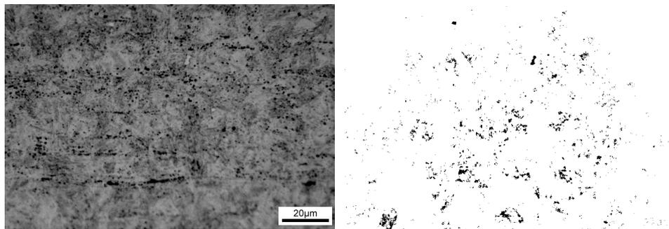
**Fig.16.** The microstructure of 15B22 heating to 880°C and sending to the mold in 20 seconds after die quench.
