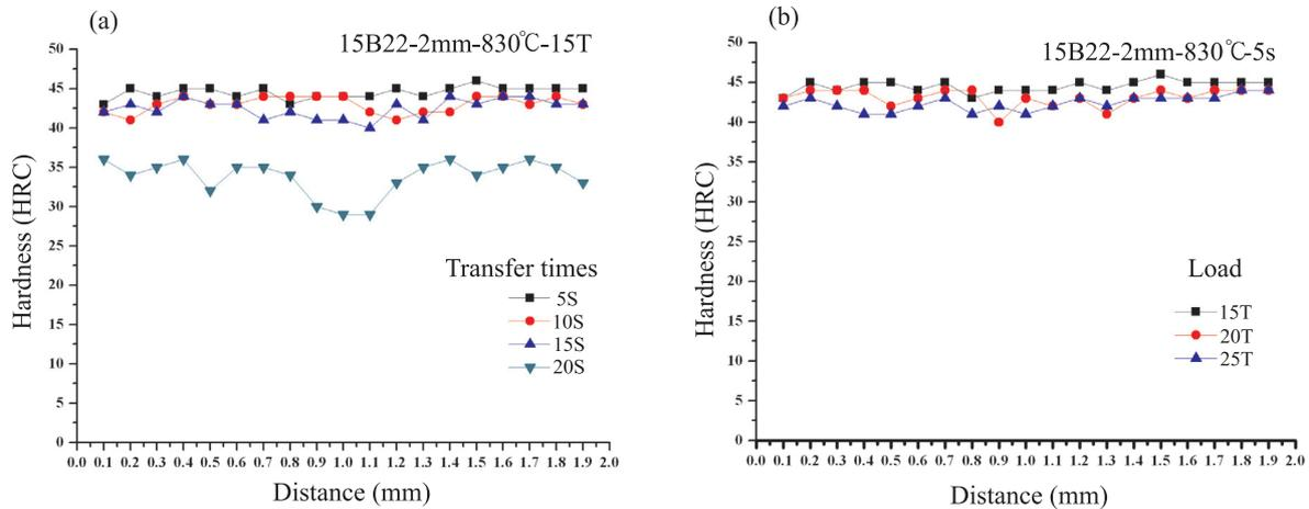
Fig.12. Hardness of 15B22: (a) for different transfer times; and (b) under different pressures.
