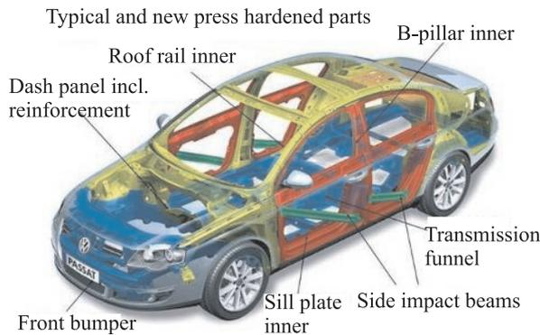
Fig.3. Hot stamping parts for automotive applications in a car<sup>(2,3)</sup>.
