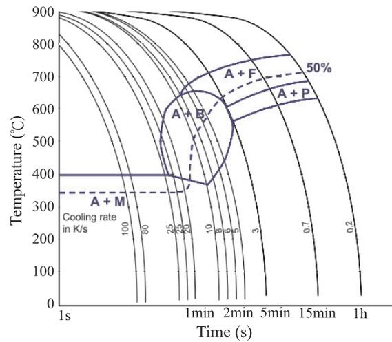
**Fig.8.** CCT curves of hot stamping process temperature vs. time with various cooling rates<sup>(6)</sup>.
