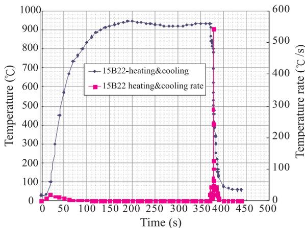
**Fig.7.** Curves of heating and cooling temperature as well as instantaneous rate of 15B22 as heating to  $930^\circ\text{C}$  followed by cooling after transferral to die quench.
