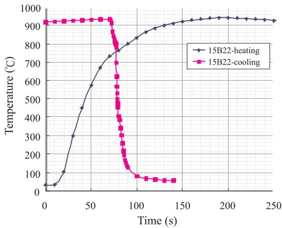
**Fig.6.** Curves of heating hot stamping steel of 15B22 ( $t = 2\text{mm}$ ) to  $930^\circ\text{C}$  and that of cooling after die quench.
