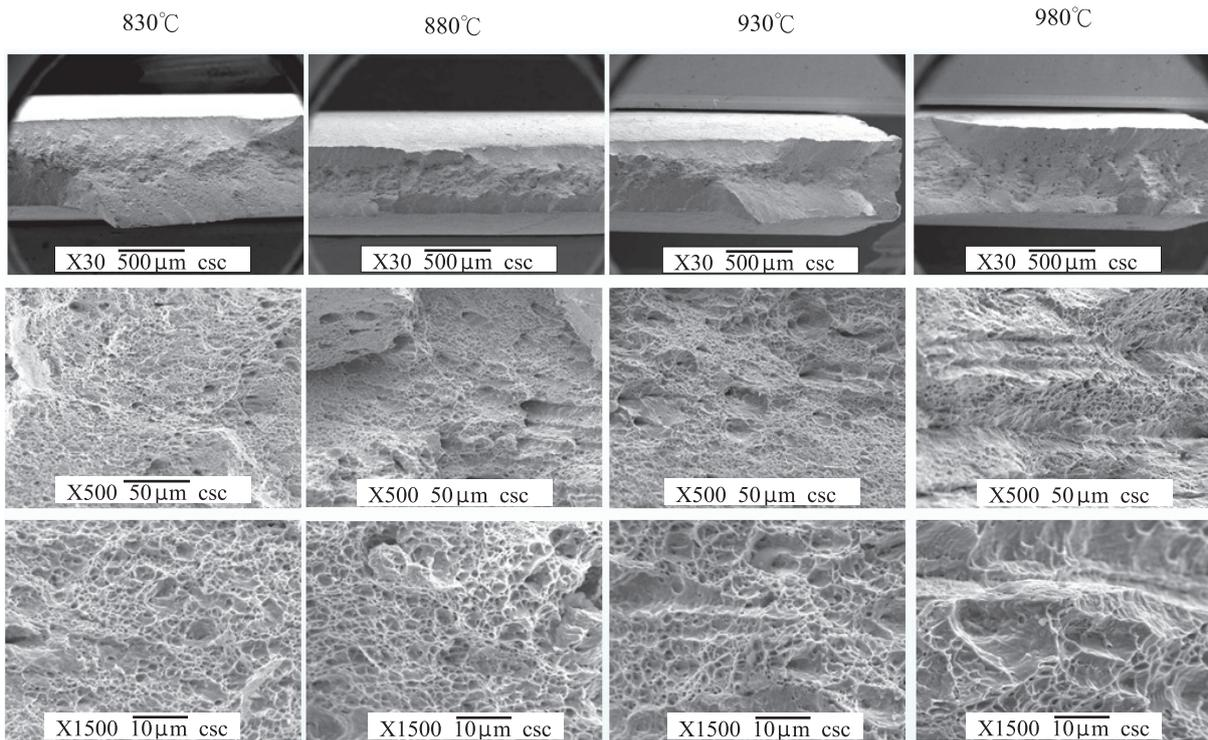
**Fig.14.** SEM analyses of cross-sectional tensile specimens of 15B22 after die quench.
